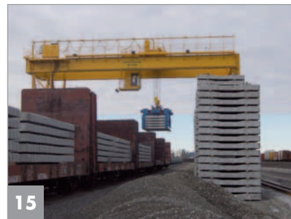
Finishing the production process: cutting of ties, application of clippings for the rails, transport and storage
