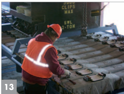
Finishing the production process: cutting of ties, application of clippings for the rails, transport and storage
