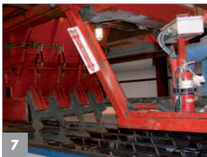
Concrete handling and filling of moulds
