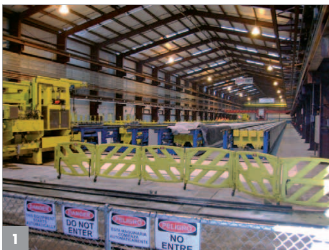
Each of the four prestressing beds is capable of producing 180 concrete ties.
